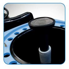
The unique anti foam device dramatically reduces the foam generation and prevents it from touching the suction motor, thus protecting its operation. The electronic floating switch stops suction when the tank is full.
